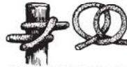
The clove hitch is used for making a line fast temporarily to a pile or bollard.
