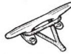
An eye spliced into the end of the line provides a convenient method of making it fast to an open cleat.
