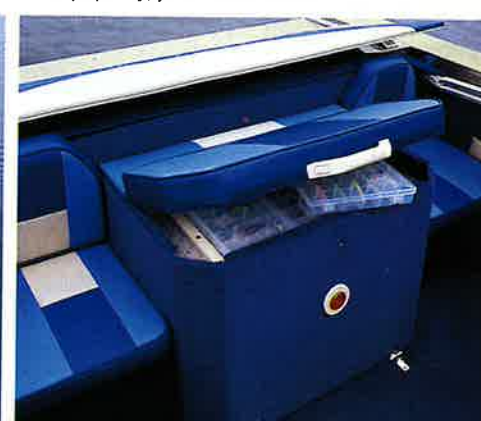
Easy access removable tackle trays and top-hider are integrated into the I/O motor box.
