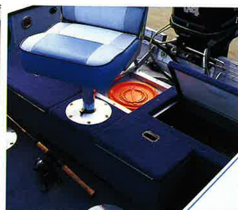
An aft casting platform makes more room for fishing and storage.
